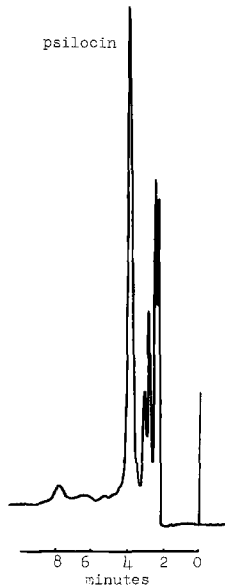
FIG. 2—Chromatogram of extract from dry mushrooms, on a 30-cm \mu Bondpak C18 column with a 40:60:0.15 (v/v/w) methanol/phosphate buffer (at pH 7.2)/cetrimonium bromide eluant.
